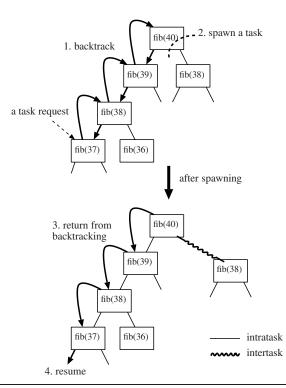
**Figure 5.** Spawning a task lazily while computing fib(40). When a Tascell worker detects a task request (at fib(37)), it (1) backtracks to the oldest task-spawnable point, (2) spawns a task for fib(38), (3) returns from backtracking, and (4) resumes its own computation.
