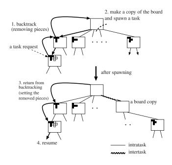
**Figure 6.** Spawning a task lazily while performing backtrack search for Pentomino. Unlike in Figure 5, (1) the backtracking step includes undo operations (i.e., removing pieces). (2) The spawning-half-iterations step includes making a copy of the temporarily restored board. (3) The returning-from-backtracking step includes redo operations (i.e., setting pieces).
