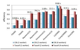
**Figure 13.** Efficiency with multiple workers in a shared memory environment within one node. Efficiency is defined as  $S/n_w$  where S is a speedup to a sequential C program and  $n_w$  is the number of workers. (Efficiency = 1 means an ideal speedup.) The number above each group of bars shows the execution time in C.
